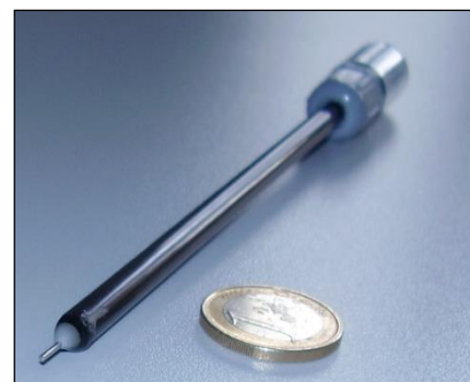
Redox electrode with S7 laboratory plug
