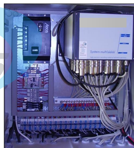
Data logger unit for 18 redox electrodes, temperature sensors and many others
